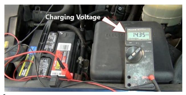
6. The next step is to load test the alternator to see if it can hold up under heavy usage. While the voltmeter is still hooked up and the engine still at a raised RPM turn the headlights and air conditioner on full. This will demand an electrical system load which will force the alternator to perform to its maximum output. If the voltage starts to drop the unit is weak and needs replacement.
