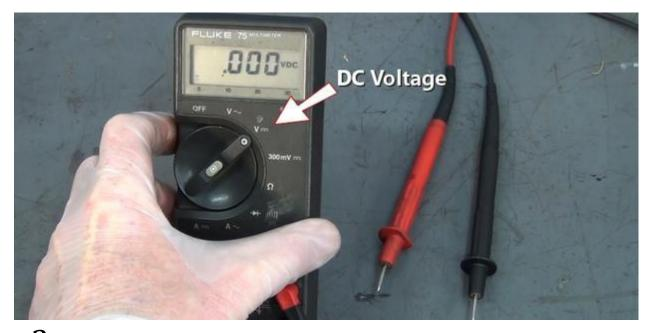
2. Locate the battery which is under the hood in most cases but some car's have them under the back seat or in the trunk. If you have a set of alligator clips that came with your meter you can change them out for the standard point probes which make testing easier but are not necessary. You can simply hold the test probes to each one of the battery terminals during the test. Wear gloves and protective eyewear.
