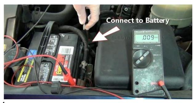
**4.** The voltmeter should read the battery voltage @ about 12.2 to 12.6 volts. If the battery is down on charge these readings will be lower and can be anywhere from 6.5 to 10.8 volts. If so the battery will need to be load tested, charged or replaced before testing can begin.
